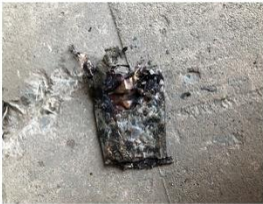
Exploded Lithium ion battery.
